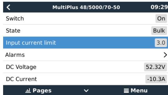
The limit as set by the user in the Cerbo GX will be applied to all inputs where 'Overruled by remote', configured with VictronConnect or VEConfigure, is enabled:
