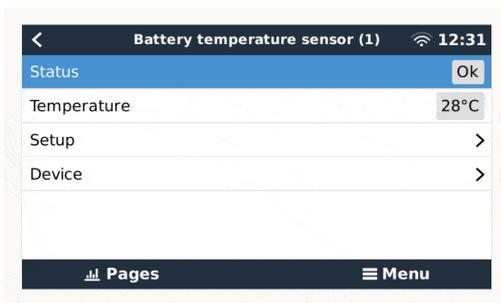
It is possible to adjust the temperature offset and scale, however for now this feature is limited to users with 'superuser' permission level.
