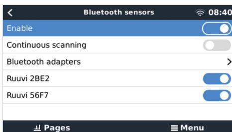
The Bluetooth adapters submenu displays a list of available Bluetooth adapters. The menu option Continuous scanning permanently scans for new Bluetooth sensors.
