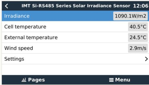
Within the 'Settings' sub-menu it is possible to manually enable and disable any optional/additional external sensors that are connected to the IMT Si-RS485 Series irradiance sensor.
