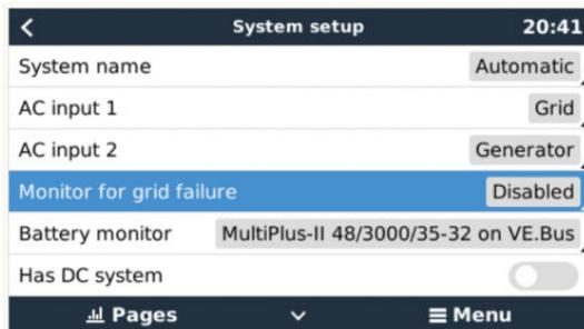
The alarm shows as a Notification in the GUI, and as an alarm on the VRM Portal, and is available on ModbusTCP / MQTT.
