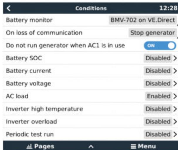
\* **Battery monitor:** Select how the battery will be monitored - if at all. The battery monitor data will be used for DC-related conditions.
