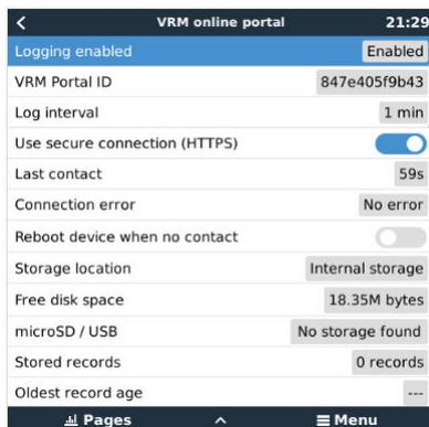
The transmission of the data logs has been designed to work also on bad internet connections. Lines of up to 70% permanent packet loss are still sufficient to get the data out, even if delayed in some cases.
