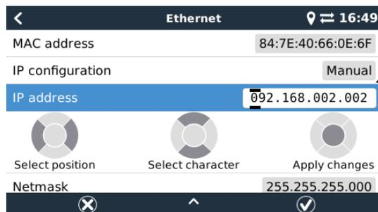
Complete details of IP requirements, as well as used port numbers will be found in the [VRM FAQ - ports and connections used by the \[82\] Cerbo GX](#)
