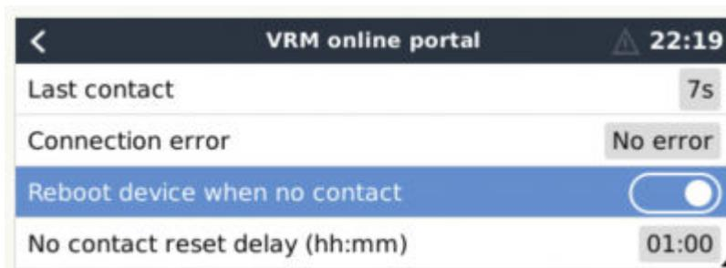
This feature, disabled by default, makes the GX device automatically reboot itself in case it has not been able to connect to the VRM Portal.
