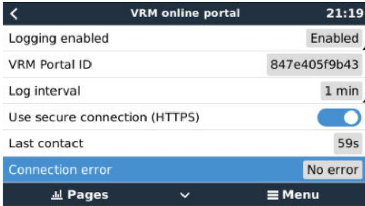
If a Connection error is shown, the Cerbo GX is not able to contact the VRM database. The connection error will show an error code that indicates the nature of the connectivity problem. Also, details of the error message are shown, to facilitate on site IT experts to diagnose the problem.
