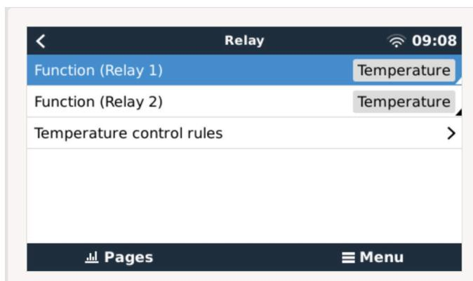
Each temperature sensor can be used to control the relay.
