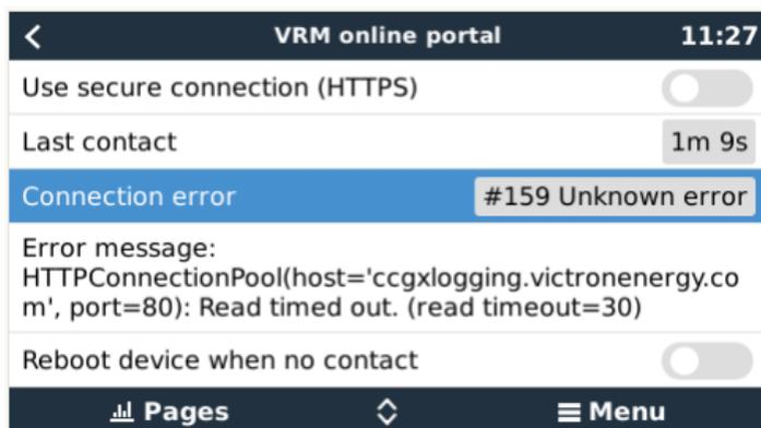
Check 'Last contact'. If this shows dashes, the GX device has not been able to contact the VRM Portal since power up. If it shows a time, but still an error is shown, then the GX device has been able to send data, but has since lost contact.
