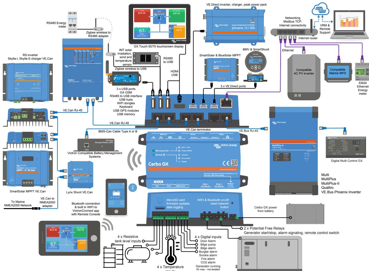
On the Cerbo GX, the USB socket closest to the HDMI connector can only be used to power a GX Touch. That USB port can **not** be used for any data related functions such as VE.Direct to USB cables, USB-sticks, USB-GPS-es, or other common USB usages. It's a power port only, no data.
