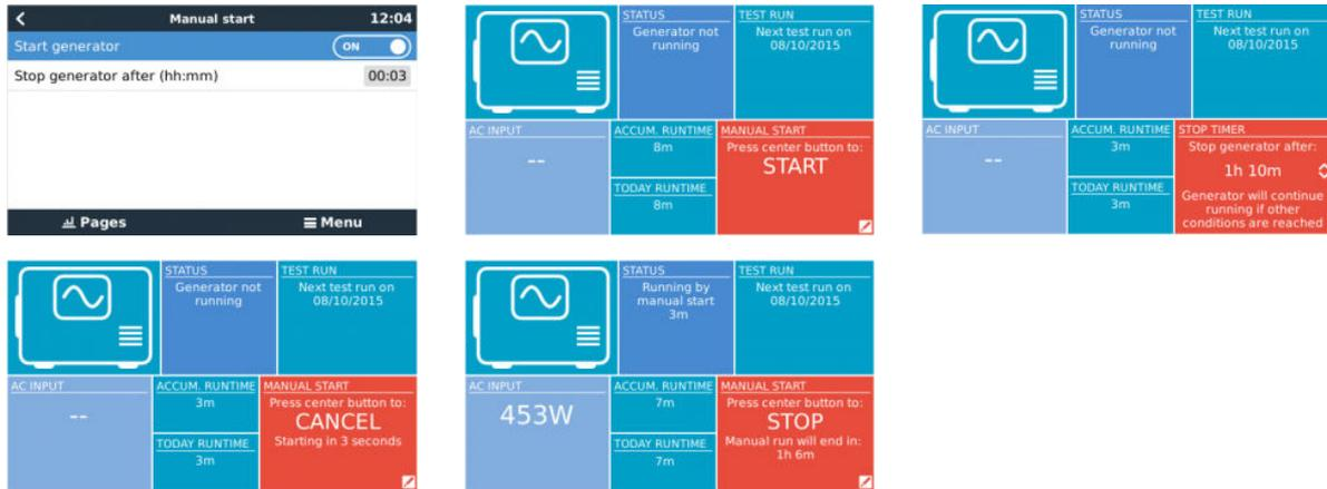
**WARNING:** If the generator is started manually (remotely) without using the stop timer, it will run until the 'Off' button has also been manually toggled.
