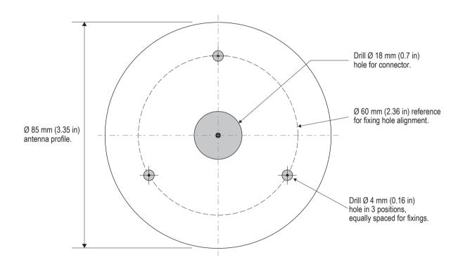
NOTE: This document may NOT print true to scale. Before modifying mounting surface, ensure printed template matches the measurements provided.
