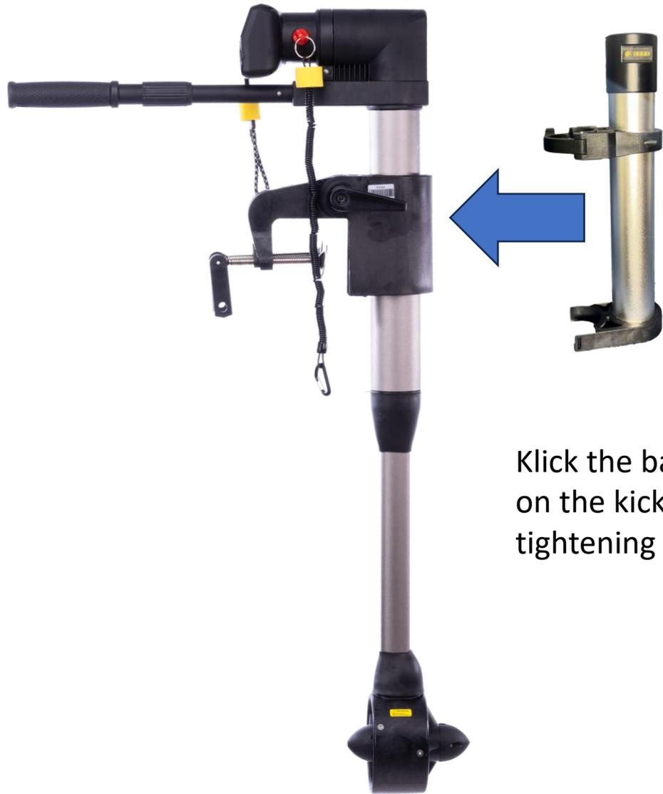
Click the battery on the back on the kicker and fasten the tightening screw
