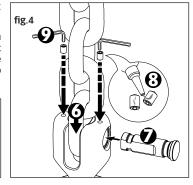
threadlocker to the short M4 dowels dowels until they stop the pin from sliding (fig. 4).
