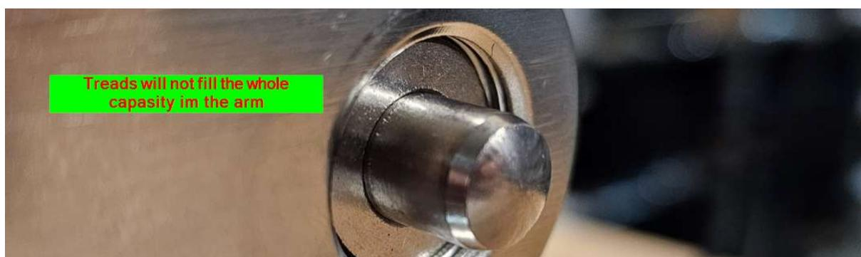
Once you have established the optimum position, lock the device with Loctite and contra nut. Always lubricate threads before making up. Test and adjust to perfect lock function before final locking of the threads.
