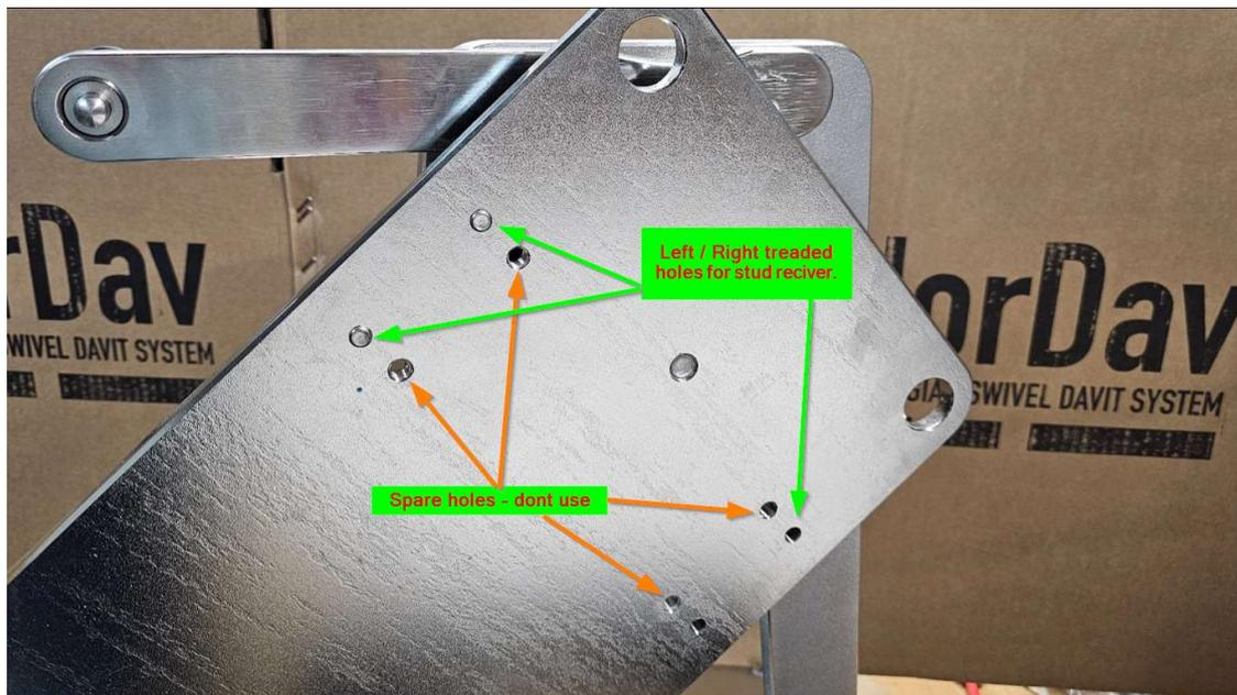
All treads need to be lubricated prior to assembly, lubrication may be replaced by locking compound such as Loctite for this installation. We recommend locking all the screws with Loctite to avoid losing integrity due to vibrations in the boat.
