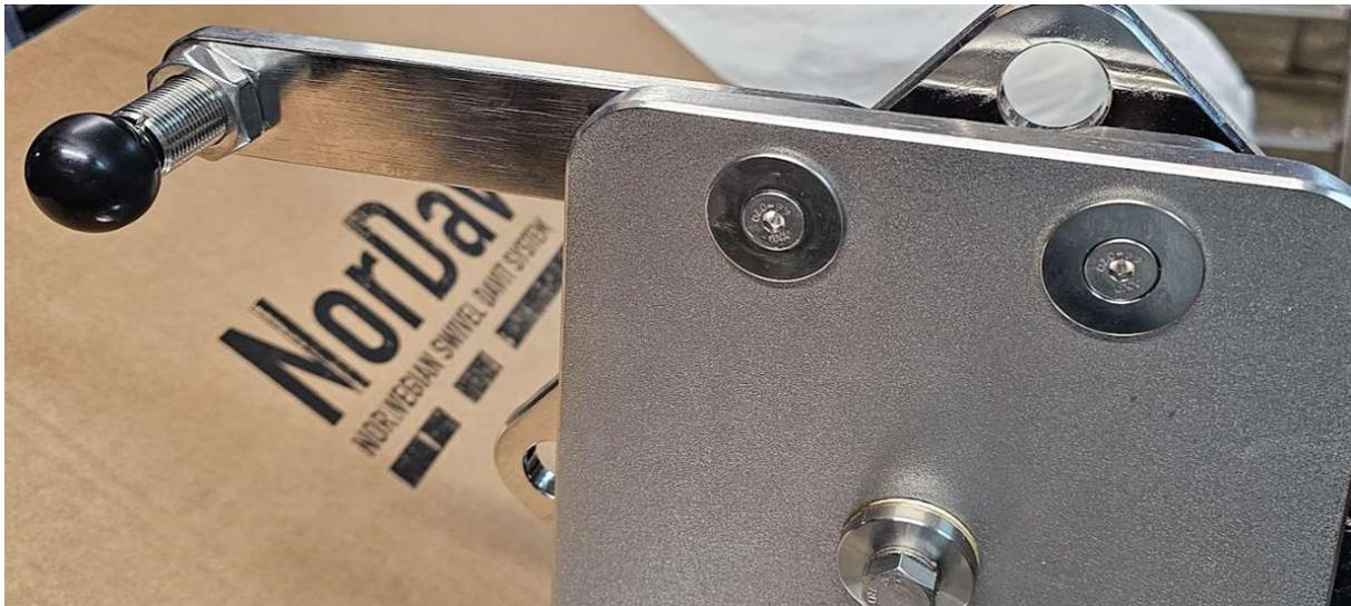
Install the lock arm with spring loaded lock. This arm can be installed both ways, by flipping it upside down and move the spring-loaded lock to the opposite side in the treaded hole.
