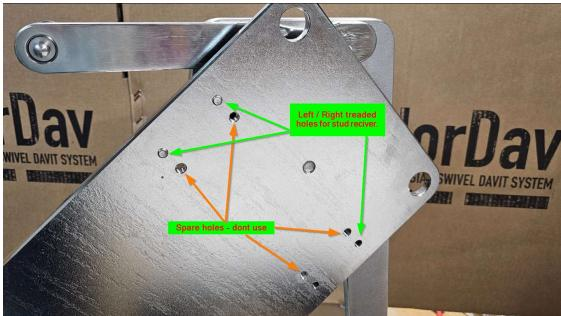
All treads need to be lubricated prior to assembly, lubrication may be replaced by locking compound such as Loctite for this installation. We recommend locking all the screws with Loctite to avoid losing integrity due to vibrations in the boat.
