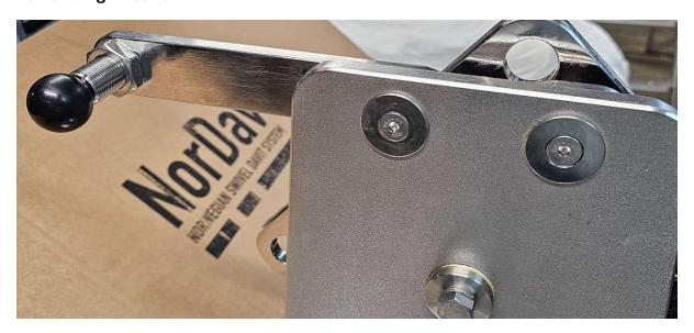
Install the lock arm with spring loaded lock. This arm can be installed both ways, by flipping it upside down and move the spring-loaded lock to the opposite side in the treaded hole.
