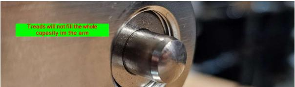
Once you have established the optimum position, loch the devise with Loctite and contra nut. Always lubricate treads before making up. Test and adjust to perfect lock function before final locking of the treads.
