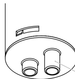
Drain hose connector  $\phi 14$
