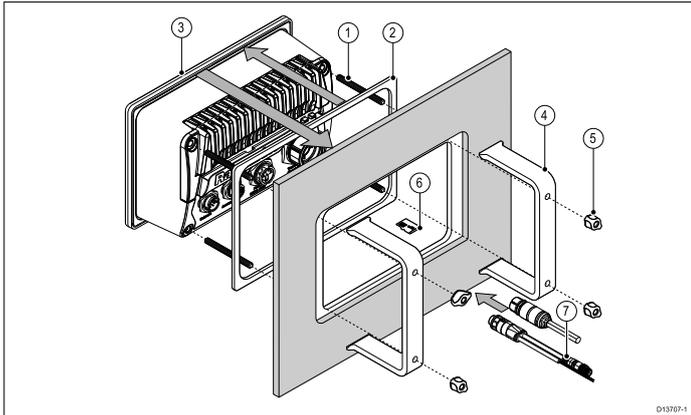
1. Screw the 4 x studs into the rear of the MFD.
