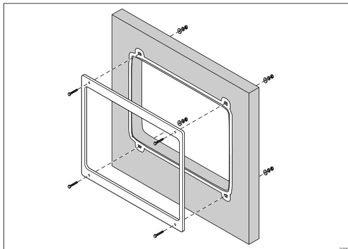
1. If supplied, center the mounting template over the existing opening, then mark and drill the new fixing holes.
