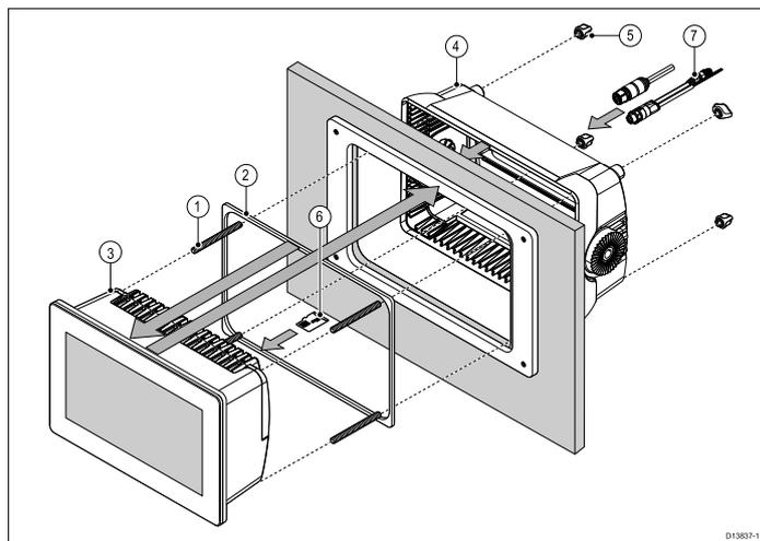
1. Screw the 4 x studs into the rear of the MFD.
