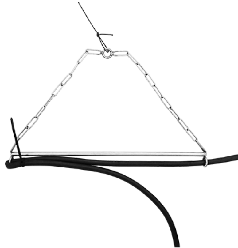
Suspension. Angle of tump illustrates how it should hang underwater. This is to stretch the hose.
