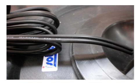
Whether the water-kit is 115V or 230V one of the pump wiring has writings on it. This wiring has to be connected on «L» while the other one on «N».
