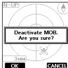
**TIP**: You can also stop the MOB mode by selecting the "Stop MOB" item on the Menu screen.
