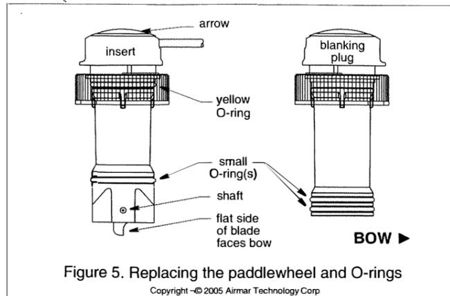
weeks. Clean the insert with a Scotch-Brite® scour pad and mild household detergent, being careful to avoid scratching the depth transducer. If fouling is severe, remove the paddlewheel (see step #1 below). Lightly wet sand it with fine grade wet/dry paper.
