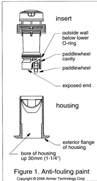
Figure 1. Anti-fouling paint
