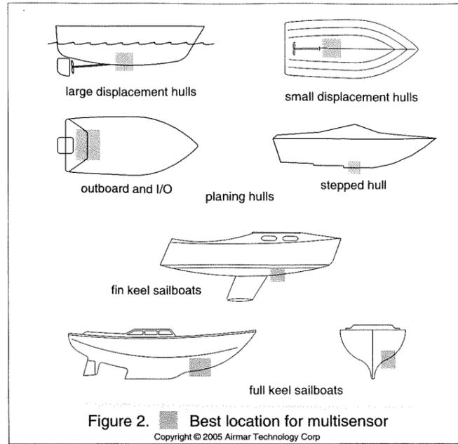
Figure 2. Best location for multisensor
