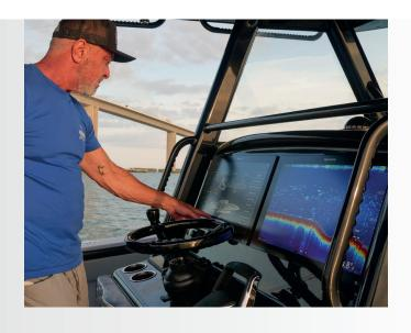
Axiom displays with radars, sonar modules, IP cameras, and Teledyne FLIR thermal cameras. The RNS-5 also supports networking with Raymarine YachtSense digital control systems and the YachtSense Link marine mobile router. Two RNS-5 switches can be daisy-chained
