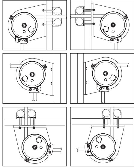
The mounting bracket allows the user to install the windlass in a variety of combinations.
