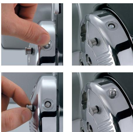
The **Automatic Free-Fall System** applied to the Balder windlass allows free running of rope through the gypsy when lowering the anchor; simply by depressing the down control button the windlass will release its clutch and the gypsy will freewheel. To stop the Free-Fall depress the up control button on the windlass; the clutch will engage stopping the gypsy and allowing retrieval of the rope. The Free-Fall function can be bypassed to facilitate power controlled release.
