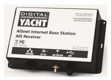
Digital Yacht has developed a new AIS receiver appropriately named AISnet which has been designed specifically for use as an AIS shore-side base station.
