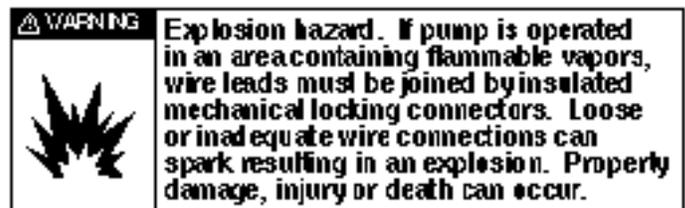
THE "WARNING" PLACARD SUPPLIED WITH BLOWER MUST BE MOUNTED ADJACENT TO ENGINE IGNITION SWITCHES (ALL LOCATIONS) TO COMPLY WITH TITLE 33, PART 183; SUBPART K, USCG VENTILATION REGULATIONS. \*
