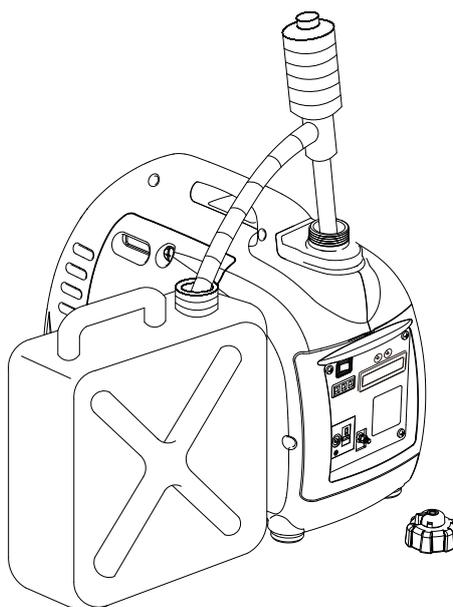
b. Turn the engine switch to "ON" position, and loosen the carburetor float bowl drain screw to discharge from inside of carburetor float bowl.
