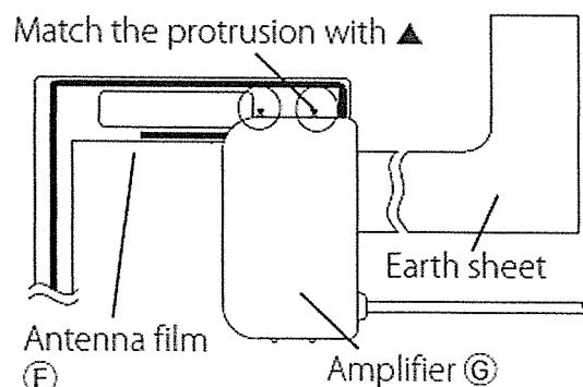
When installing the antenna on the left side
