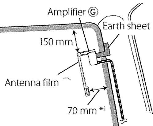
\*<sup>1</sup> Where the earth sheet of Amplifier G can be pasted on the metal part of the front pillar.
