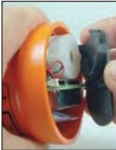
5. Remove old O-ring (using for example a plastic card). Use Vaseline (acid free) and fit a new O-ring in place.
