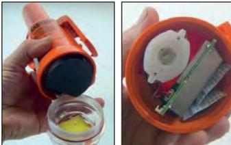
3. First, pull out the battery then pull out the cable from the connector.
