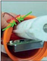
2. Connect the cable to the electronics (black = left & red = right)
