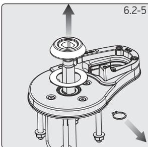
Assemble the new gypsy in reverse order, note that the part number engraved on the stripper ring should face upwards.
