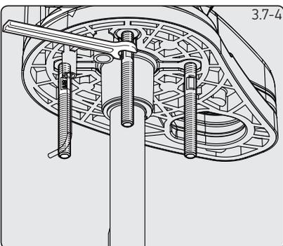
4. Assemble and tighten studs into base until they bottom out in their holes. Some studs have a flat. Position the flats of the studs nearest the base of the windlass.
