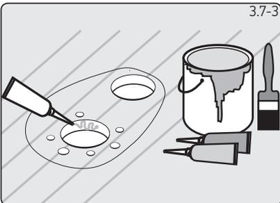
3. When all the holes have been made, remove the template. To help avoid water absorption by the deck, apply an appropriate marine sealant to the freshly cut hole edges.
