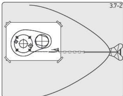
2. Using your template and after you have checked all the above and below deck requirements cut the following holes.
