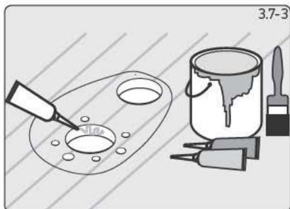
3. When all the holes have been made, remove the template. To help avoid water absorption by the deck, apply an appropriate marine sealant to the freshly cut hole edges.
