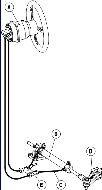
Single station + lock valve
