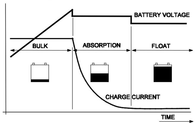
Three-stage charge curve: Stage A: BULK, for quick charging from 0 to 80%, Stage B: ABSORPTION, the battery is charged from 80 to 100%. Stage C: FLOAT, battery is maintained in fully charged state.
