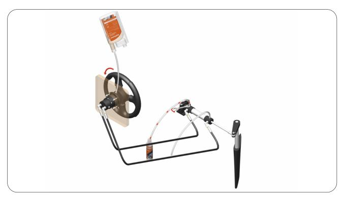
**STEP 16:** Continue to turn the Steering Wheel towards Starboard Side. When the Oil comes out from air bleeder without air bubbles then carefully close the air bleeder. Do not overtight the air bleeder. Continue to turn the Steering Wheel in the same direction to fill the Cylinder chamber. During this phase, the Cylinder body will move to the opposite direction up to the end stroke.
