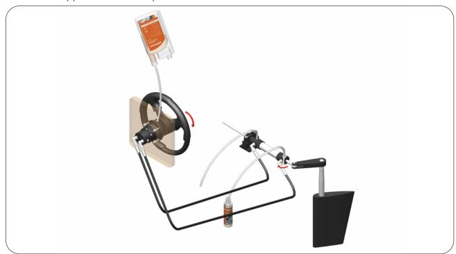
**STEP 15:** Turn the Steering Wheel slowly towards Starboard Side, so that the Oil can come out of Hoses. Unscrew the air bleeder as shown and allow the air & Oil (air bubbles) come out from air bleeder.
