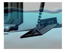
Trim tabs for small boats are also available, and highly effective for performance enhancement. These self-adjusting trim tabs work independently and require no operator interface. Automatic trim tabs are available from Nauticus with nitrogen gas-filled actuators. Nauticus trim tabs (SMART TABS®) are available in seven different models
