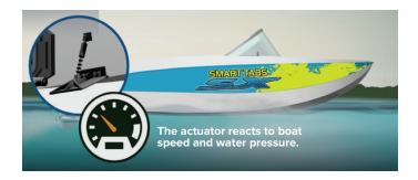
SMART TABS are self-regulated trim tabs that automatically adjust, as required, to maximize boat performance. The system is constantly active. SMART TABS use a nitrogen gas actuator encased in an air- and water-tight neoprene rubber boot. The actuator reacts to boat speed and water pressure to adjust the trim plate angle and control the amount of lift.
