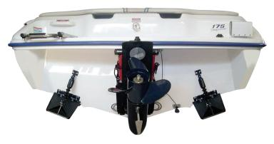
Automatic trim tabs are available from Nauticus with nitrogen gas-filled actuators.
