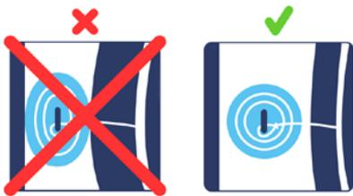
As with classic fenders, you should not position POP Fenders in places where plastic film – for whatever reason – is attached to the hull. Rays of sunlight can heat up this film, which can then result in being rubbed off by the fender.
