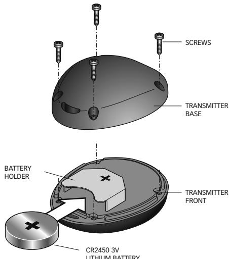
**WARNING:** once the transmitter is assembled, verify that the LED does not remain on constantly. If the LED is on, reopen the transmitter and verify that it was assembled correctly.
