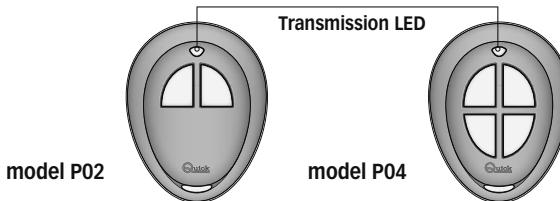
**WARNING:** the transmitter needs to be programmed in the receiver's memory. To do this, follow the procedure shown in the receiver's user manual.
