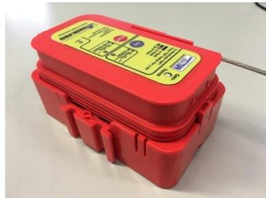
Place the vmsTRACK-PRO into the Battery-Charger. The battery charger must be connected to DC power supply (9 to 32 VDC, 2 A).
