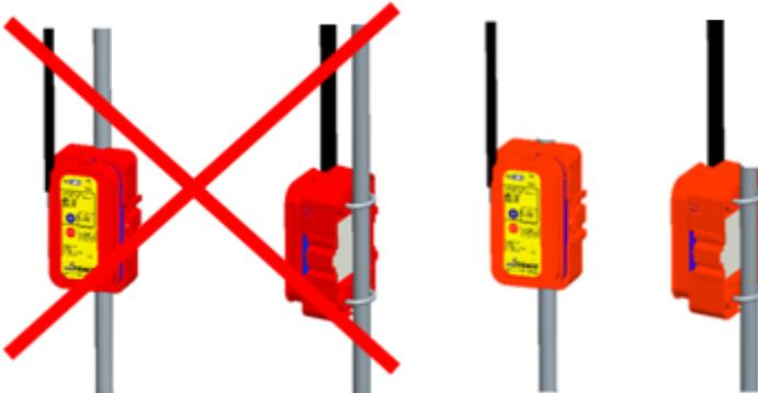
*ATTENTION: Do not have a metal pole close to the antenna (left figure). This would significantly reduce the radiated power of the VHF signal. The right figure is perfect.*
