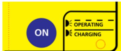
In charging mode (i.e. the unit was turned off before) the yellow LED is illuminated continuously during charging period.
