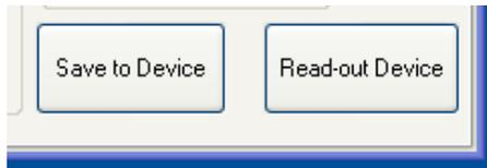
For programming and setting up the vmsTRACK-PRO device, you have to press the "Save..." button. All the settings, which were made in the "Administrator" page, will be stored into the vmsTRACK-PRO and double checked again. You will see that with the green marks.
