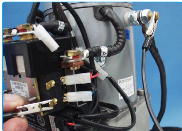
Jumping ground to blue on D2 coil
