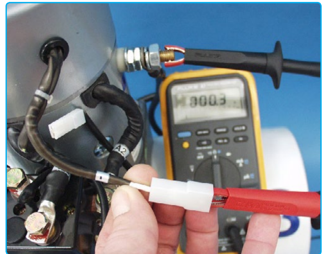
Checking continuity between negative lead and battery negative post
