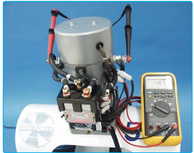
Checking voltage at thruster
