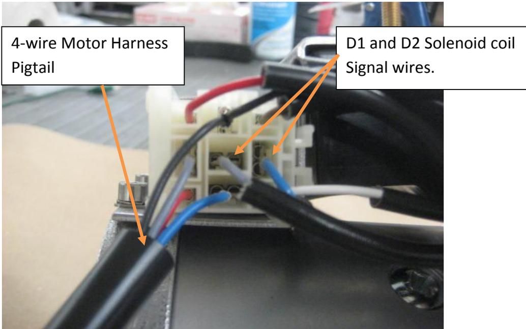
Step 4: Jump to the A1 Negative Battery Stud as in the trouble-shooting guide. If the motor does not run, verify input voltage on the Solenoid Positive Feed Terminal and check output voltage on the A2 Terminal.
