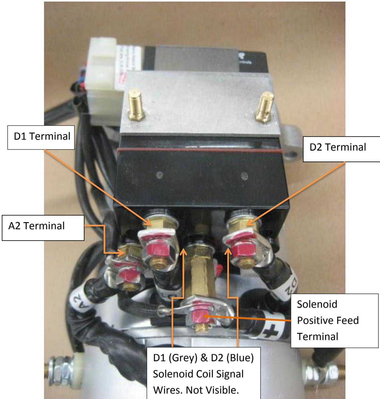
Step 1: Since the White IPC wire cannot easily be disconnected unplug the control box instead. The control box fits very tightly in the plug so it helps to wiggle it back and forth to remove it.
