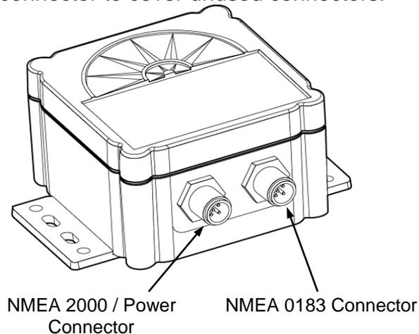
**Figure 3 – NMEA 2000® / NMEA 0183 Interface Connector Locations**
