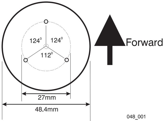
Mounting: Drill 3 x Holes (size depends on the material being drilled)
