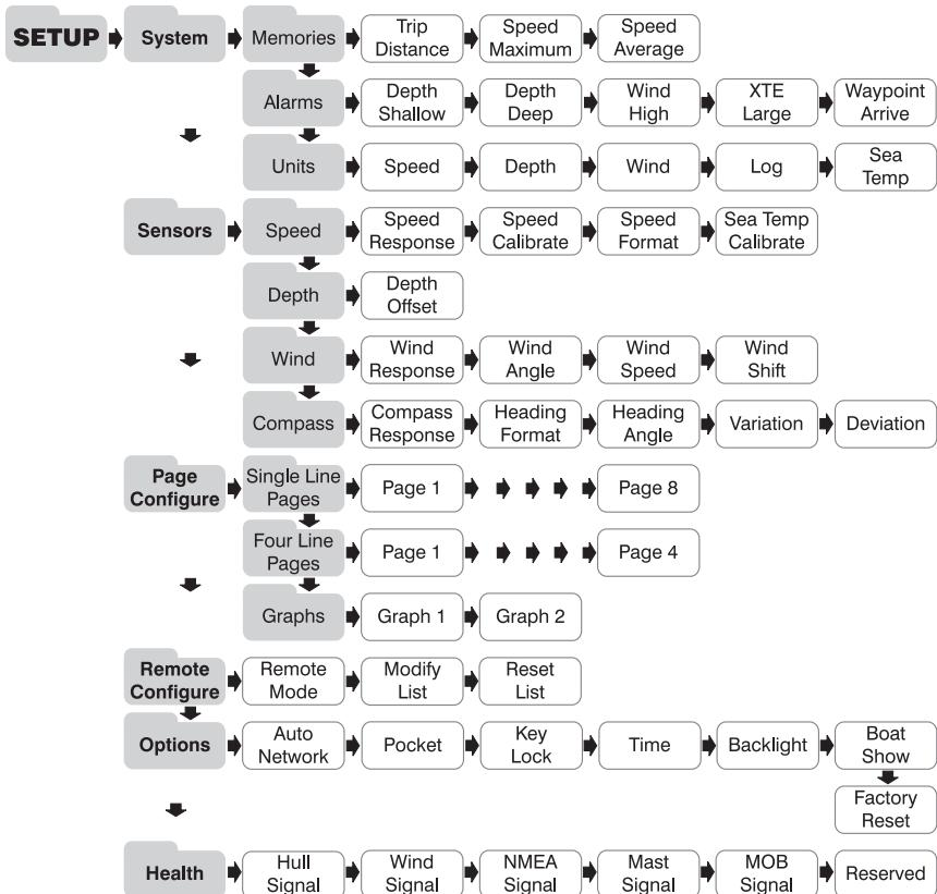
**To enter the Setup and Calibration menu:** press and hold the button for 2 seconds. A list of chapters is displayed, with the active chapter marked with the cursor .
